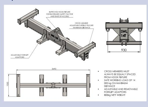
The adjustable spreader beam is able to withstand loads of up 14 metric tonnes and can be customised for each client's exact requirements.
